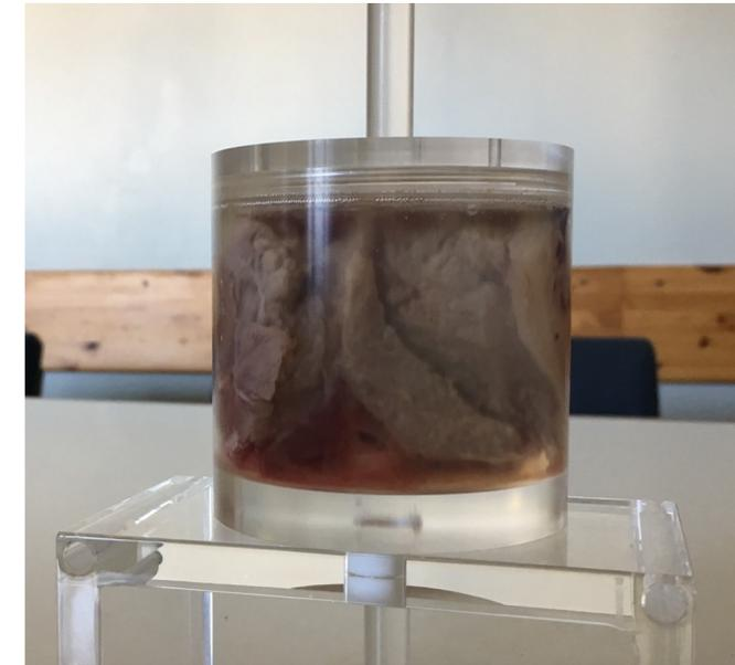
Direct proton range measurement phantom
