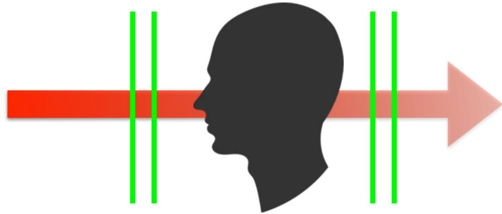
Total deflection-angle squared determined for each proton based on measurements of spatial position in each of the four tracker units. Total mean-square angular deflection can be approximated as:
