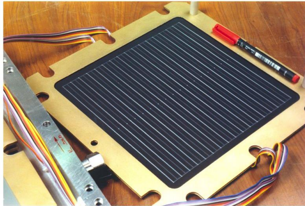
The segmented IC in the standard IBA nozzle uses 32 strips instead of pads, with another 32 orthogonal. The dosimetry pad has to be on a separate plane. A Monte Carlo study showed this would also work, and it cuts down on the electronics.
