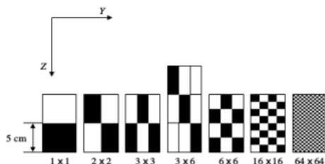
Figure 1. Illustration of density heterogeneities studied in this work. The black areas represent the compact bone through which the proton beam passes upstream of the water phantom, and the white areas represent air. The adopted coordinate system is also illustrated. Geometries are plotted on the plane  $x = 0$  cm. The beam axis was in the  $z$  direction.
