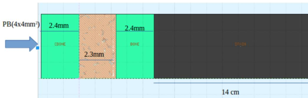
**Figure:** Modelled phantom having 2.3mm trabecular bone sandwiched in between two(2.4mm each) layers of hard bon.
